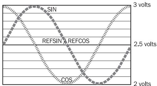
Diagrams Signal specification of the process channel
