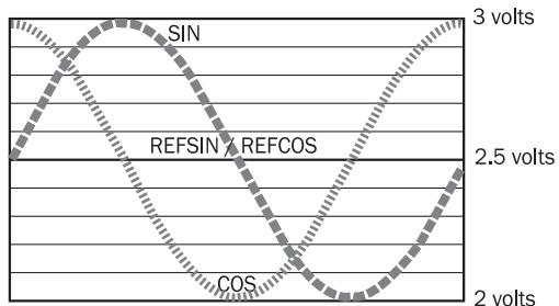
Diagrams Signal specification of the process channel
