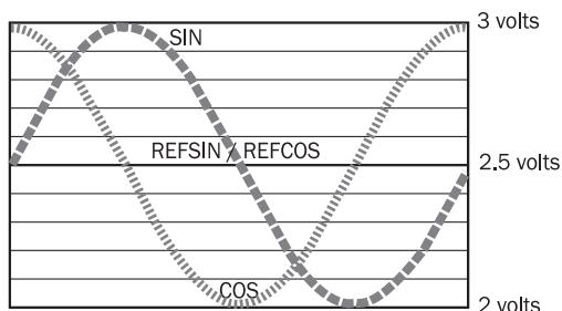
Diagrams Signal specification of the process channel
