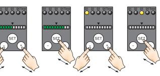
Position object in light field. Press SET button > 1 s. If requested adapt tolerance with
