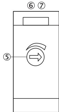
⑤ Sensing range adjustment: potentiometer, 5 turns
