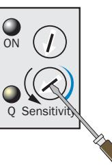
If yellow LED illuminates, turn "Sensitivity" rotary switch counter-clockwise until the yellow LED just goes out.
