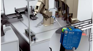
Ideal for use in mounting technology thanks to precise detection Reliable quality control thanks to high repeatability - even if the and distance measurement
