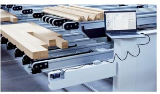
**Easy commissioning, integration and maintenance via IO-Link** Smart Sensors with IO-Link generate and receive data as well as information that goes beyond conventional switching signals or measured process parameters.
