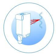
For uneven, shiny, reflective and even jet black objects, Twin-Eye technology offers a high level of operational safety. Two receivers in one sensor ensure a high detection reliability. Find out more in the video
