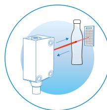
In the case of transparent objects such as glass bottles or cling film, the ClearSens technology guarantees reliable detection results.
