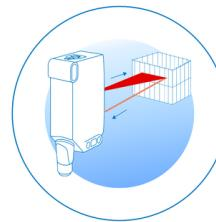
The LineSpot technology offers a high detection reliability for perforated, structured and uneven objects.
