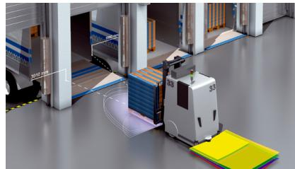
For instance, the MRS1000 simplifies quick and collision-free entry into a truck by detecting and monitoring the driving path.
