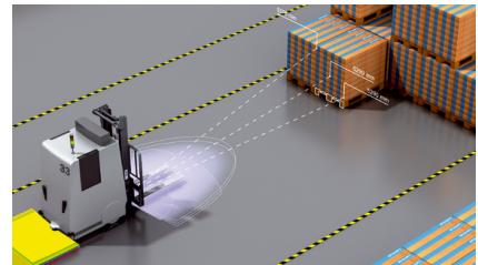
The MRS1000 allows for correct positioning of the transport fork of an automated guided vehicle during the approach and reception of the pallet without stopping the AGV.
