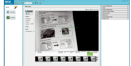
SOPAS interface, a comprehensive configuration and monitoring tool which makes possible a clear view of the read process.
