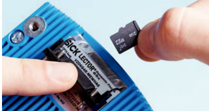
Slot for microSD memory card. Parameter cloning and storage of images.
